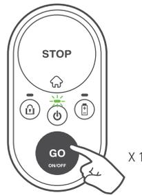
If the regular mowing duration is too long for your lawn, you can initiate a short mowing operation (of up to 60 minutes) by pressing the GO button twice.
