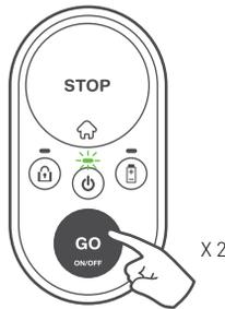
When child protection is enabled, a special combination of keys is required to start a mowing operation. Hold down the STOP button and press the GO button once to unlock the child protection for 30 seconds. The Lock indication will be temporarily switched off. Now you can start a mowing operation as described above. As soon as the mowing operation is started, the child protection will automatically relock itself.
